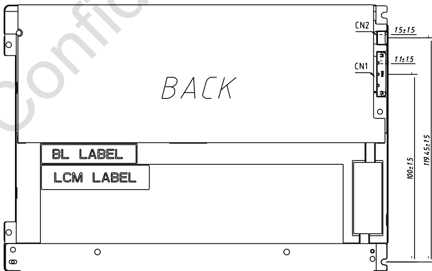
Figure 17 Reference Outline Drawing (Back Side)
