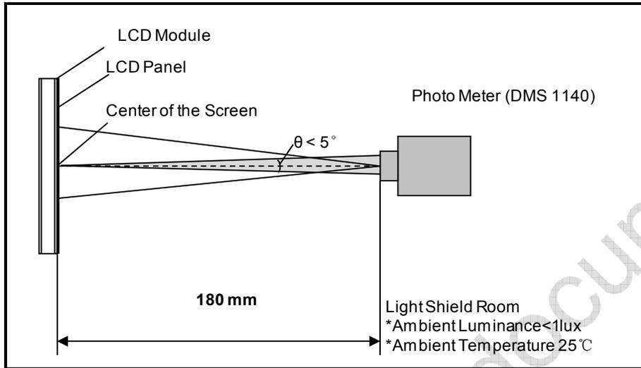
**Figure 4 Measurement Setup**
